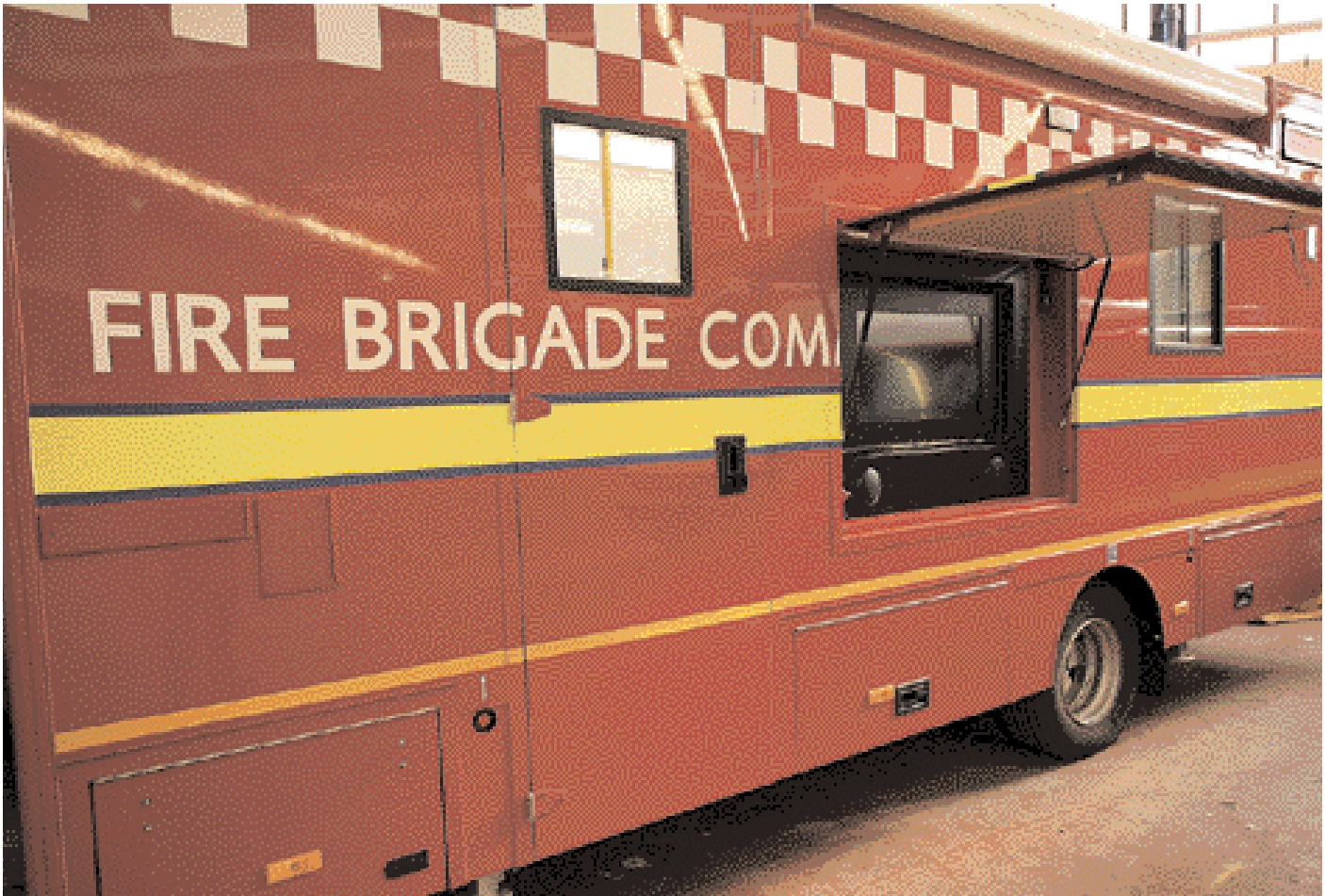
A large touch-screen mounted on the side of a vehicle allows for external briefings using the Command Support System that will not disrupt the work of the command team in the vehicle
